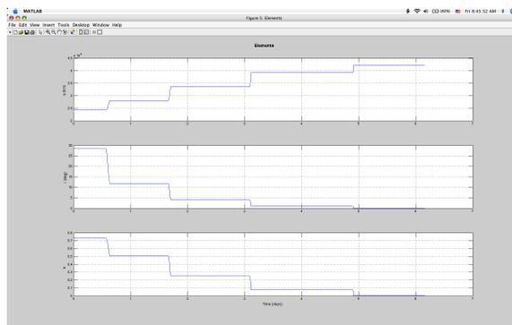
The dynamical model uses a point mass Earth model, although higher fidelity models can easily be used instead (the toolbox includes a 36<sup>th</sup> order gravity model). In this example the final burn leaves the spacecraft on station. In practice, it would be left with some drift velocity. In addition, the burn vector is held constant when small adjustments might need to be made due to orbit determination errors and orbit perturbations.
